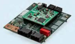
BMS Control Board
