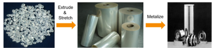
Figure 3: The extrude and stretch process. Source: TTI
