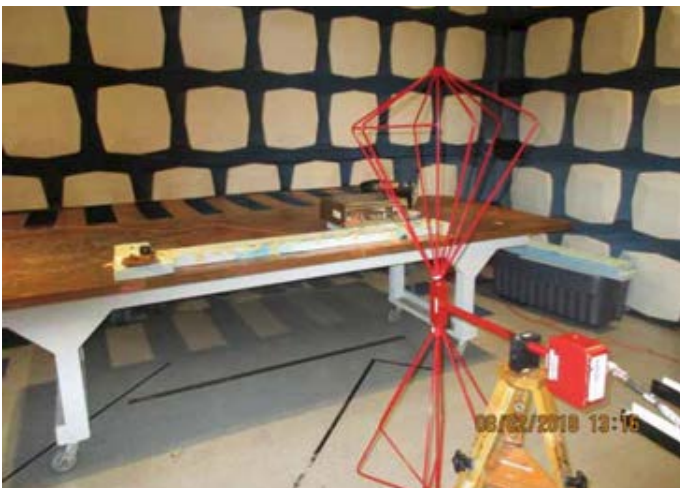
Radiated emission set-up (Vertical BICON test in a single DUT mode)
