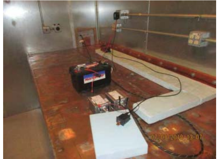
Conducted emission set-up on the power conductor.
